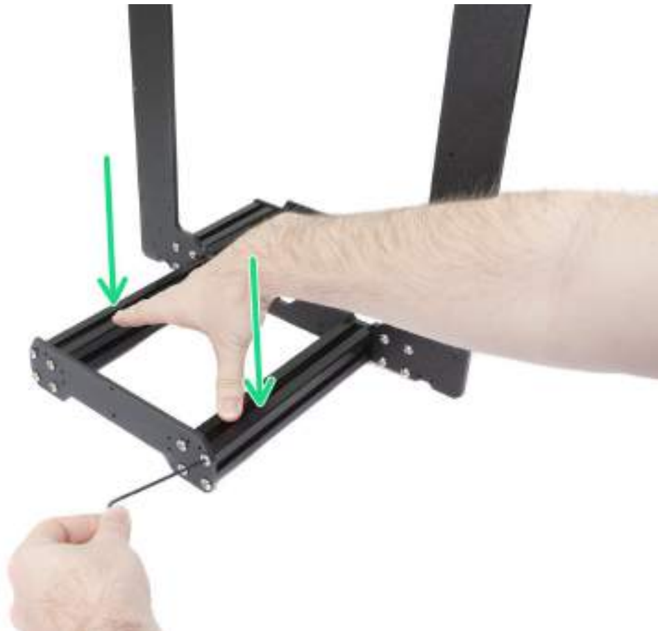
Pict. 41 - Proper way to tighten the frame, plates and aluminium extrusion together.
