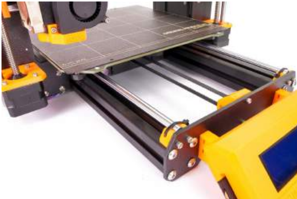
Pict. 43 - A properly-tightened Y-axis belt under the heatbed
