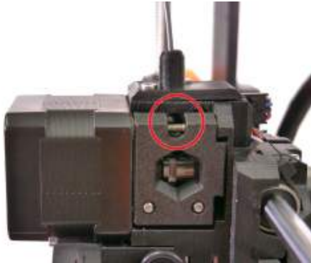
Pict. 38 - Access hole for cleaning the filament sensor
