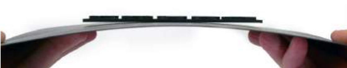
Pict. 14 - Removing the model from the PEI print surface by bending the steel sheet.
