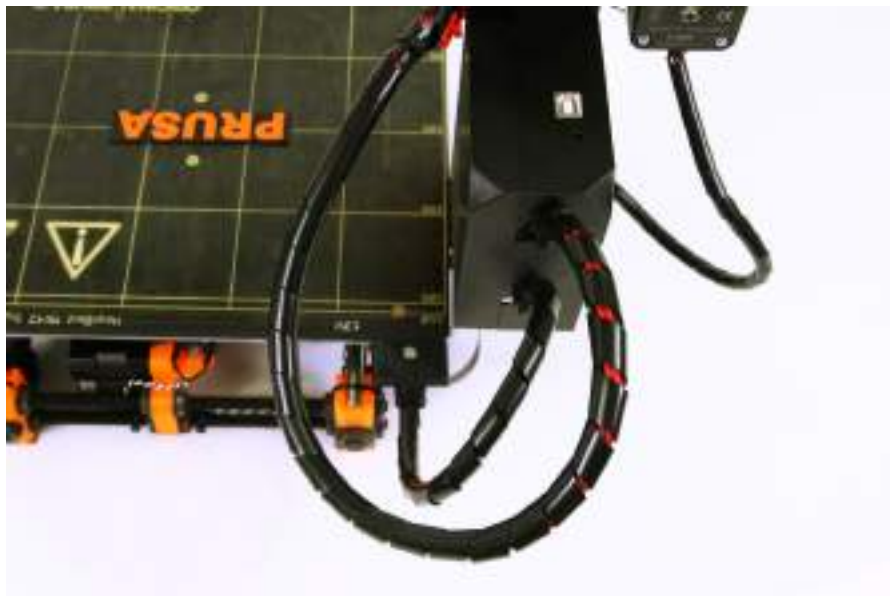
Pict. 45 - Cables should be wrapped in a spiral wrap
